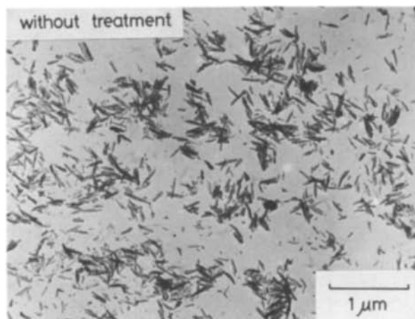
Figure 5 TEM photos of Co- \gamma -Fe 2 O 3 with and without EOS treatment in magnetic paint.
